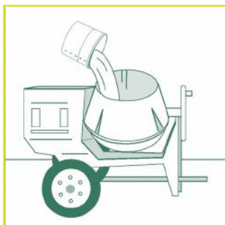
Add water to the mixer at a ratio of 3.6 litres per bag of NATCEM 35.
